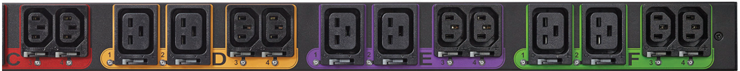
Figure 1. Color-coded outlet sections match a corresponding circuit breaker to easily identify which one feeds corresponding outlets and prevent unbalanced loading that would unnecessarily trip a breaker.
