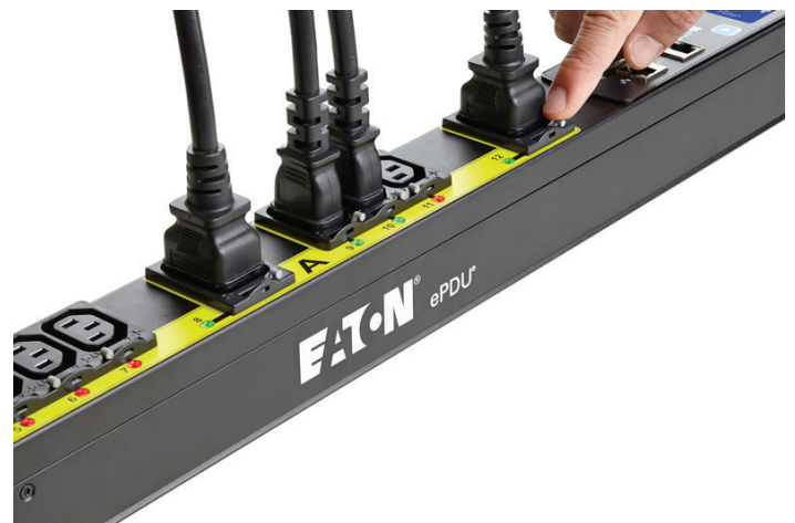
Figure 2. IEC outlet grip secures plugs in place with a lever-actuated grip that's integrated into each outlet. Once the levers click into the grip position, the plugs are secured from accidental disconnect due to bumps or vibrations without the need for special power cords.
