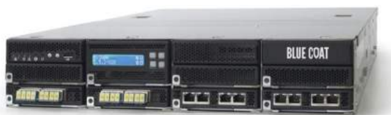
Figure 1-2: Sample SSL visibility appliance from Blue Coat.
