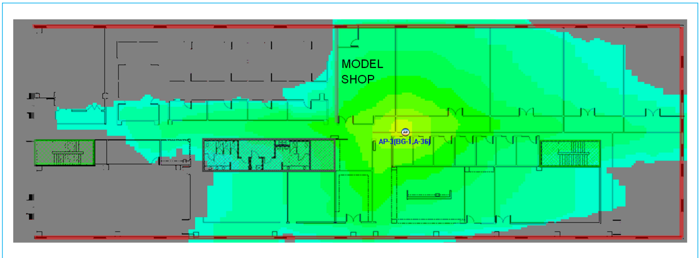
Figure 6: RF planning diagram with one access point deployed. Grey area denotes limited or no coverage.
